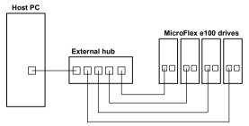
Figure 34 - Connecting to drives using TCP/IP in standard Ethernet mode
